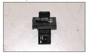
18. Install the mass air sensor into the K&N<sup>®</sup> adapter and secure with the provided hardware.
