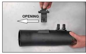
19. Install the mass air sensor assembly into the K&N® intake tube so that the opening in the sensor is towards the inlet end of the tube and then secure it with the provided hardware.
