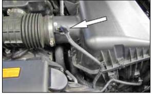
3. Disconnect the mass air sensor electrical connection and unhook the harness from the air filter housing.
