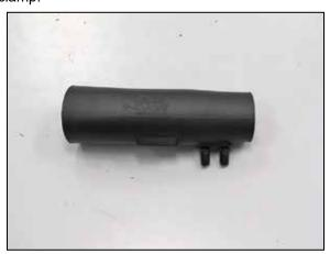
15. Install the two provided NPT vent fittings into the K&N® intake tube as shown.
