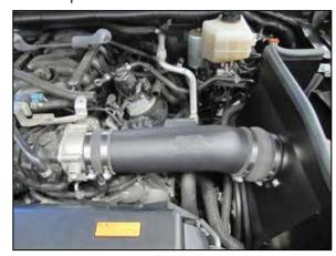
20. Install the K&N® intake tube into the hump coupler and then into the coupler at the throttle body, adjust the tube for best fit and then secure with the provided hose clamps.
